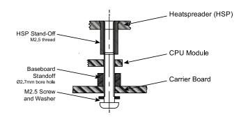
Bottom mounting scenario uses the threaded version heatspreader and requires bore hole standoffs on the carrier board.
