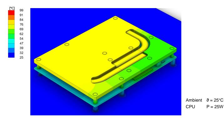
Simulation of the conga-TS170/HSP at ambient temperature of 25°C, CPU dissipating 25W of heat after a short time of operation.
